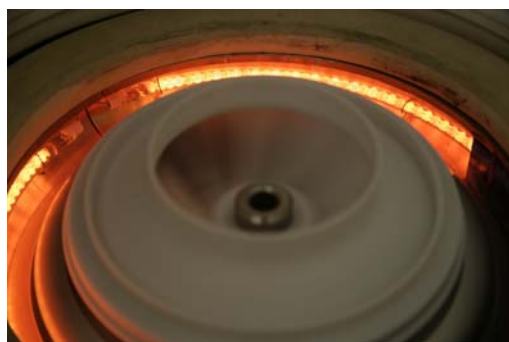
Figure 6 The rotating samples are heated using a circular high-energy IR source.
