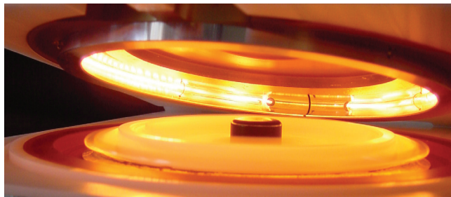
Figure 1. The rotating samples are heated using a circular high-energy IR source.
